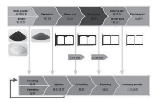
Figure 1: MIM Basic Process Flow Diagram
